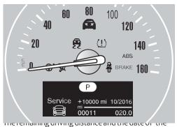
next scheduled service are briefly displayed in the speedometer immediately after you start the engine or switch on the ignition.
